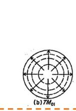
**μ = 0 is (mainly) associated to the radiation of the TM<sub>01</sub> mode in a circular waveguide.**
