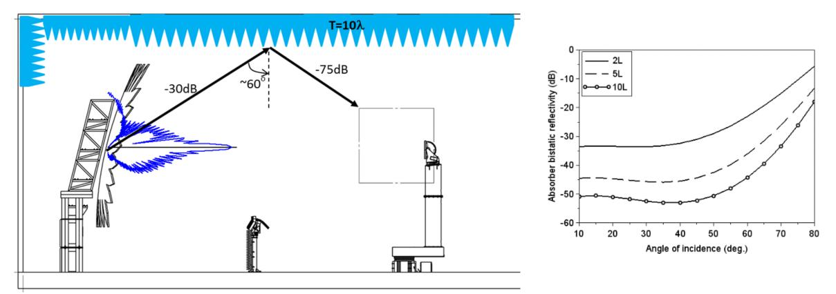
Shorter and narrower rooms increase the angle of incidence. Thinner absorber has less bi-static reflectivity.
